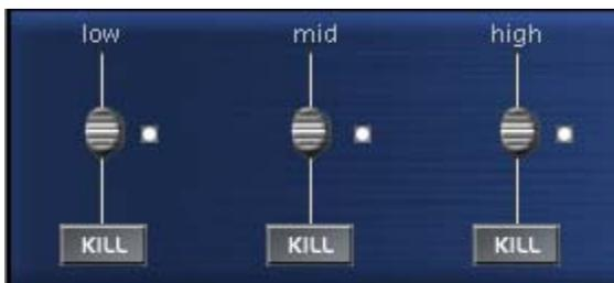
3-Band EQ Killer: Each player has 3 vertical sliders controlling Band volume and 3 KILL Buttons allowing each Band to be cut instantly.
